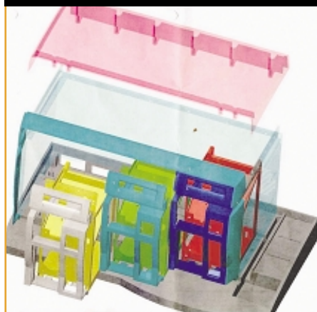
Figure 4: Modules can be individually replaced in the Fluidics Station 450
