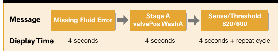
Figure 6: Diagnostic messages are displayed on the system's LCD.
